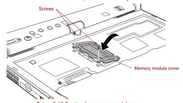
Figure 3-12 Seating the memory module cover
